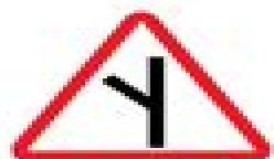
Y - intersection left
